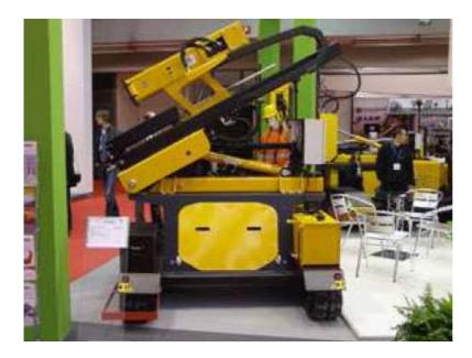
Orteco increases its range of barrier installation machines with a new compact model. At Intertraffic Amsterdam 2012 the company presented Basic, a machine which weights just 2.2 tonnes to get easier the transport from site to site.
